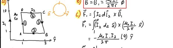
Force on filament due to loop:
